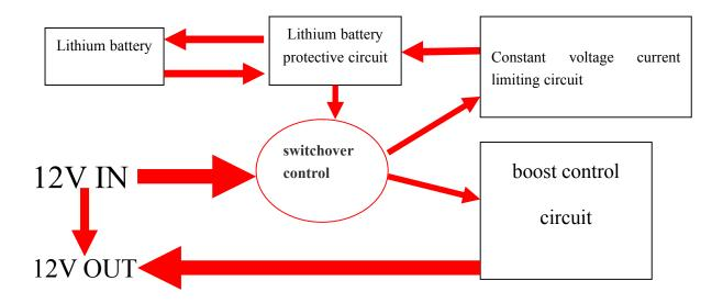
Remark: When the mini UPS switchover, there will have 10~15ms time for the voltage will drop and be less than 11V.
